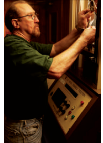
Michael Weber, responsible for quality control testing of paper, runs a tensile test.
