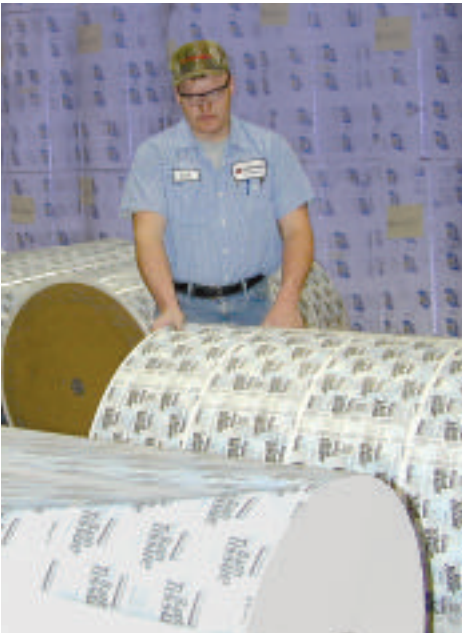
Carl Kesler prepares a printed roll for rewinding to final roll sizes at the Oconto Falls plant.
